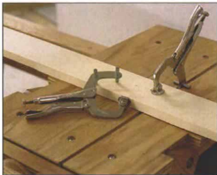
Custom clamps. Pawlik modified locking C-clamp Vise-Grip pliers by cutting off one of the swivel pads and welding two 1/4-in. rods on the jaws. The thin jaws fit into the bench-top slot and act as clamps.
