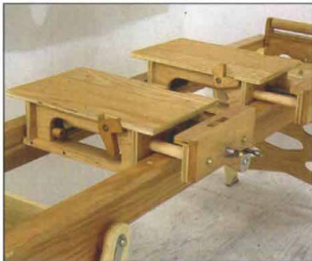
Sliding tables. Both sliding tables ride on oak runners. Each table is equipped with three bench dogs and a vise.
