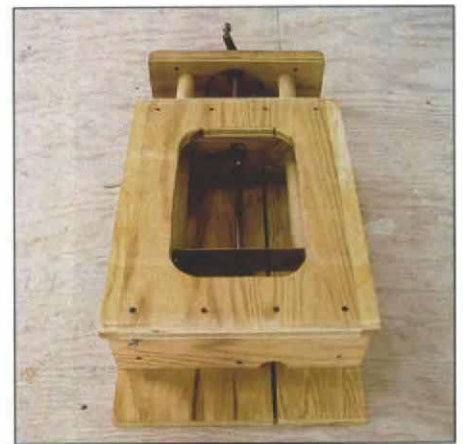
C-clamp vise. Pawlik used the screw mechanisms from large C-clamps to make the vises for the bench's sliding tables. Hardwood dowels serve as guides for the vises' jaws.
