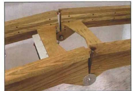
The key to rigidity. A key cut in the 1x3 sub-frame helps register and stabilize the bench's frame when it is open.
