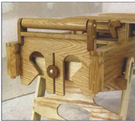
Stretchers and rollers. The stretchers are lightened by cutouts in the plywood. The outfeed rollers are held by turn screws made of a carriage bolt and a wood knob.
